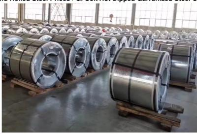
The hot dip galvalume steel is a kind of coated steel. With the cold rolled steel of different strength and thickness as substrate, it is produced through applying Al-Zn coat on both faces by hotdip process. In its coating, Al accounts for about 55%, Si 1.6%, Zn43.4%. It enjoys both the physical protective feature and durability of Al and the electrochemical protective property of Zn. Andits surface has bright silver color and regular embossed-like figure, which are highly decorative.
