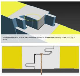
Dislocation double mortise and tenon joint provide better airtightness and free from thermal bridging benefiting from high thermal insulation
