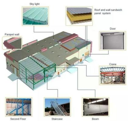
The installation of this building is incredibly easy and can be completed quickly. The steel structure is pre-fabricated, which means that it is made in a factory and then assembled on-site. This process is much faster than traditional construction methods, which can take months or even years
