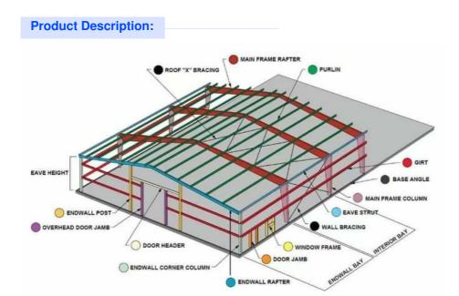
Made from high-grade Q235 and Q355 steel, this warehouse is built to last. It can withstand harsh weather conditions, heavy loads, and other types of wear and tear. This makes it an ideal choice for industrial and commercial applications where durability is essential.
